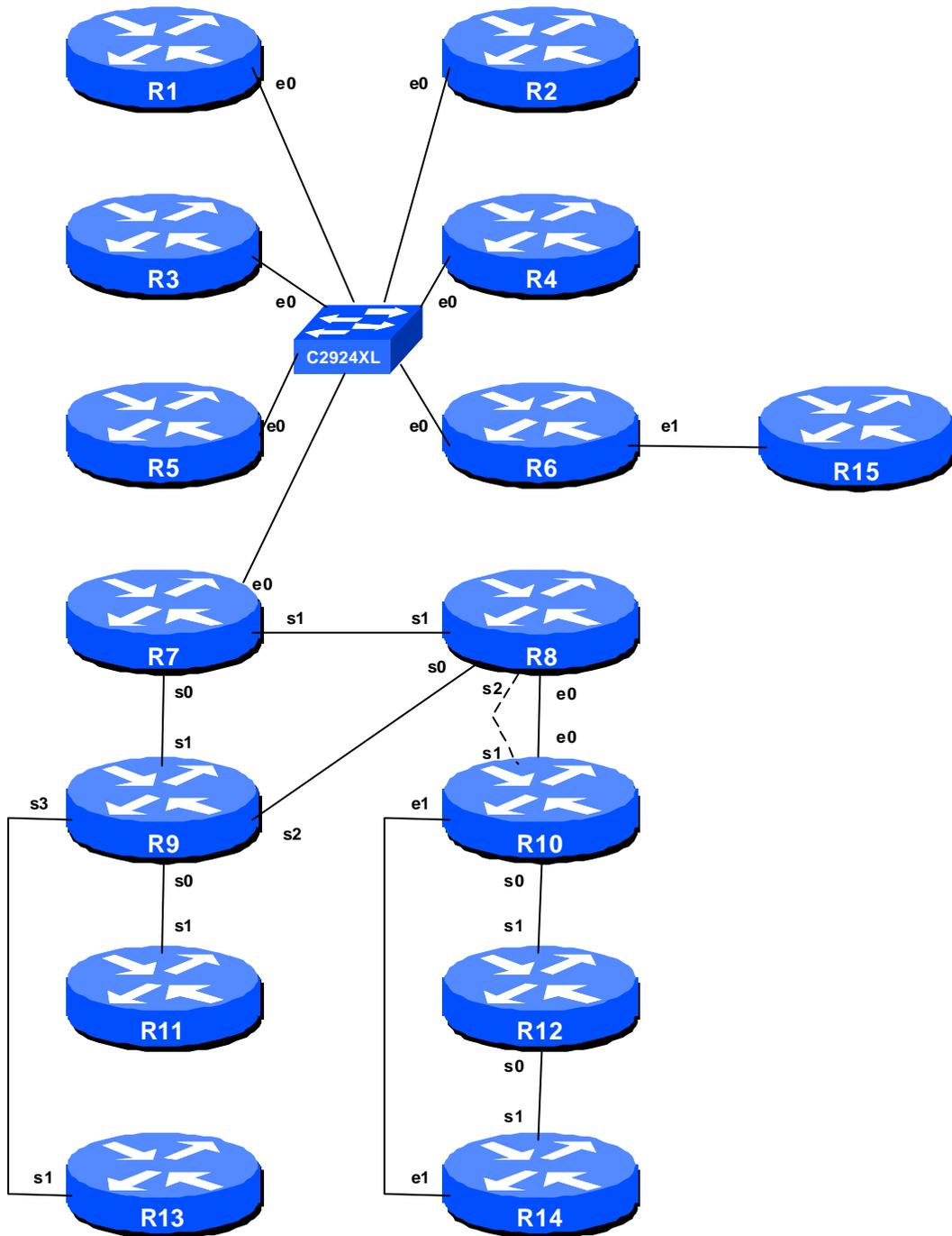
Figure 2 – Lab Physical Layout
