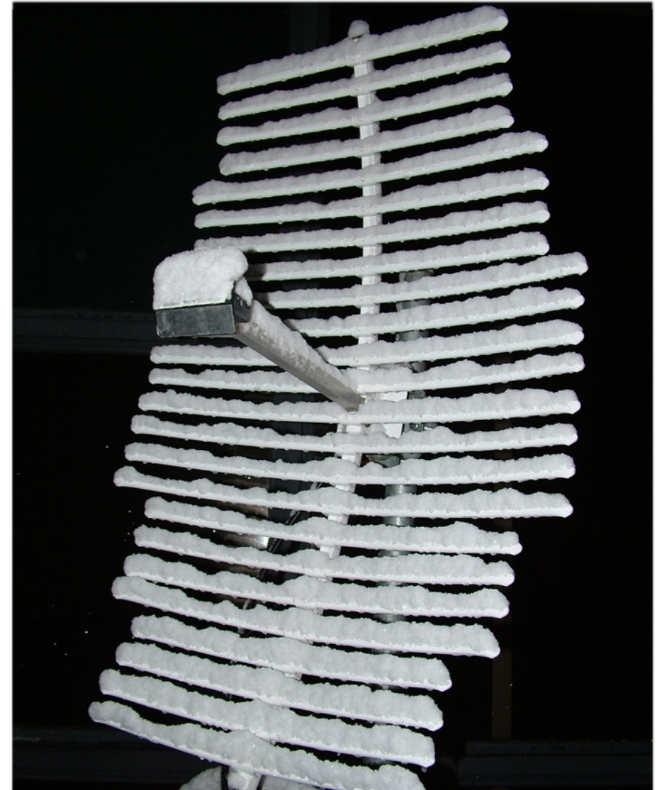
parabolic grid (covered by snow)
