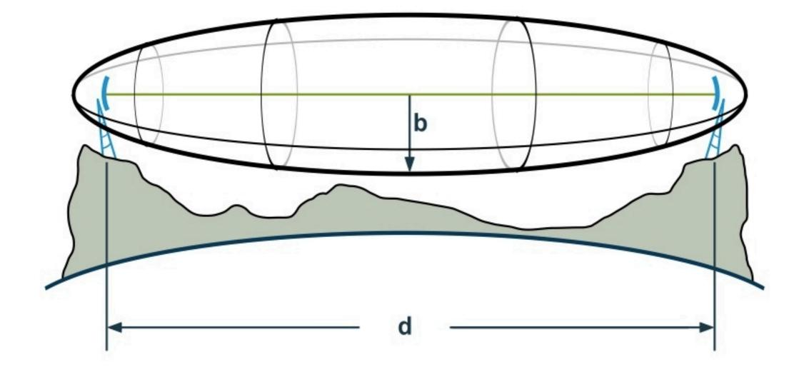
The radius of the Fresnel Zone at its widest point can be calculated as:
