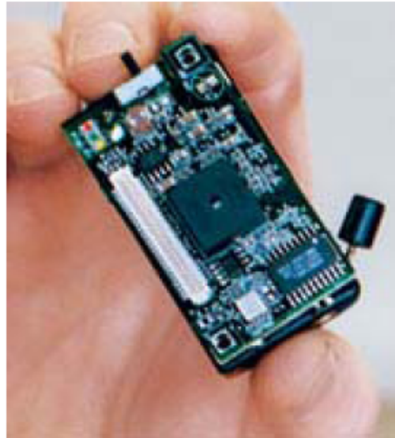
Mote maker: David Culler's "motes" monitor the environment and send reports wirelessly. (Photograph by Angela Wyant)
