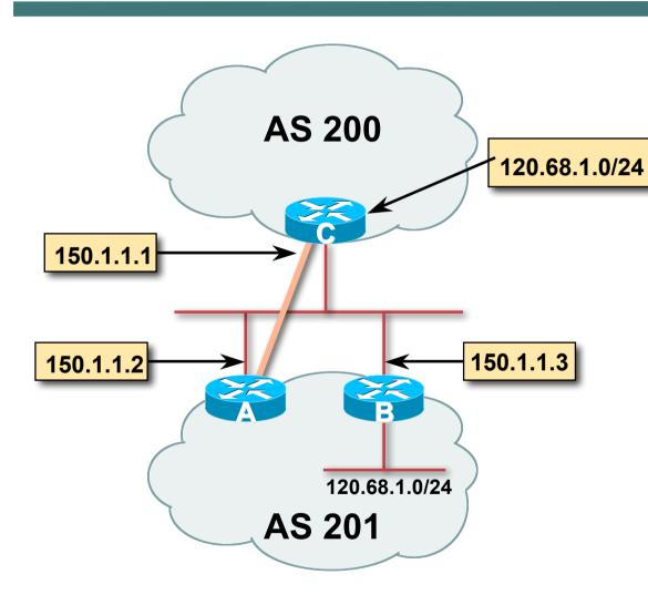
eBGP between Router A and Router C
