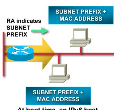
At boot time, an IPv6 host build a Link-Local address, then its global IPv6 address(es) from RA
