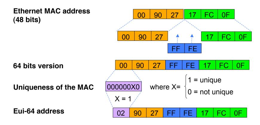
EUI-64 address is formed by inserting FFFE and OR'ing a bit identifying the uniqueness of the MAC address
